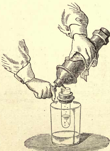
The Discharge of the Liquefied Gas.
